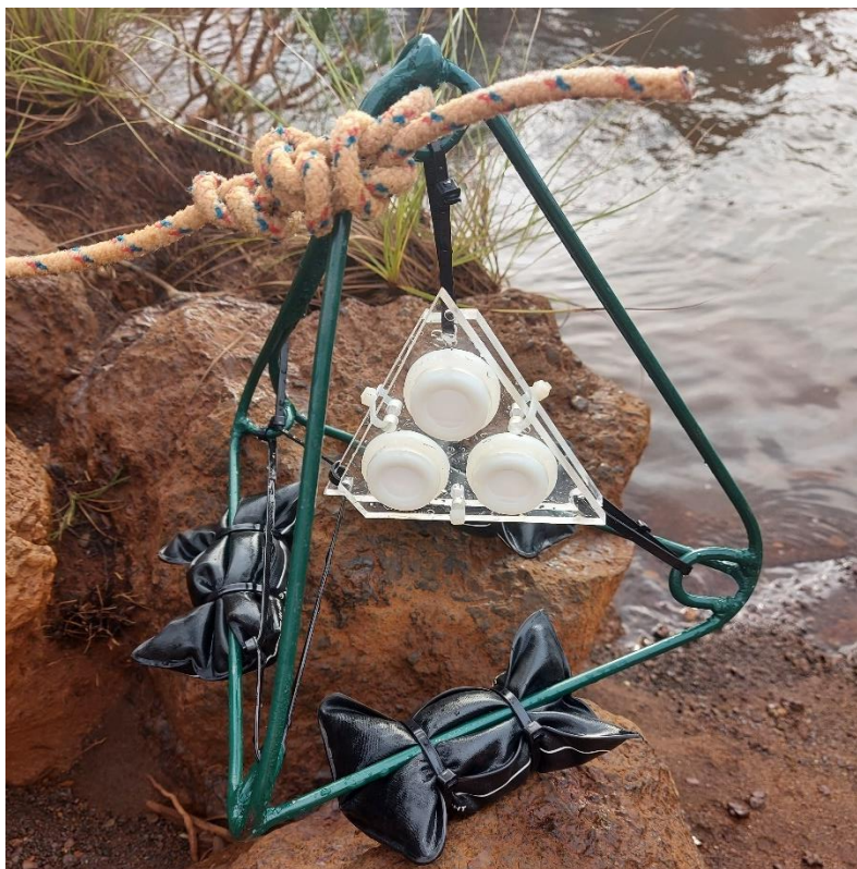
Figure 2 : Support recevant les plaquettes de DGTs.
