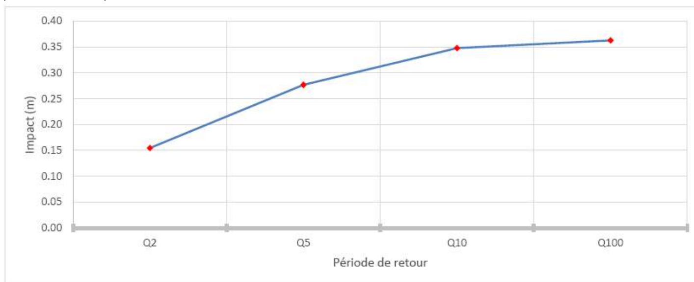
Figure 54 : Incidence maximale - obstruction partielle
