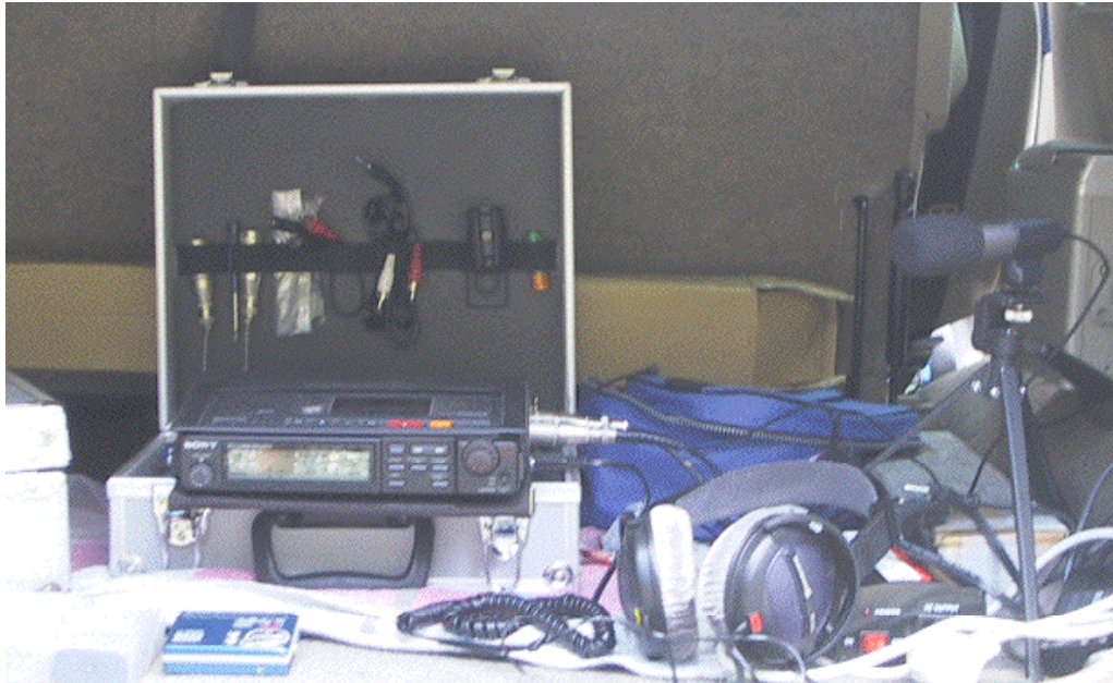
DAT (Digital Audio Tape) Sony TCD D10 PRO II Casque audio Beyer dynamic DT 911 MD digital recording Sony MZ-R70 et microphone Sony ECM-MS908C
