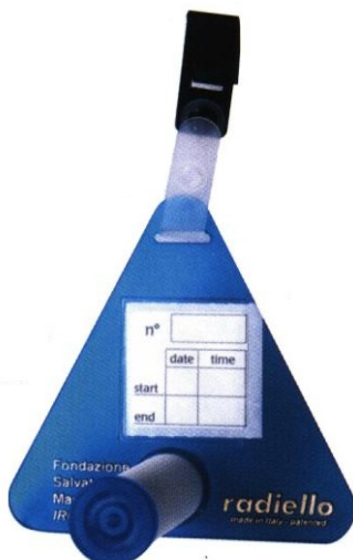
Figure 3. : Ensemble support - corps diffusif - cartouche
